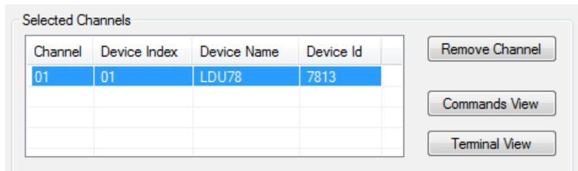
The "Terminal View" dialog is a dialog tool for sending raw parameter commands to the device and to examine the received command responses.
