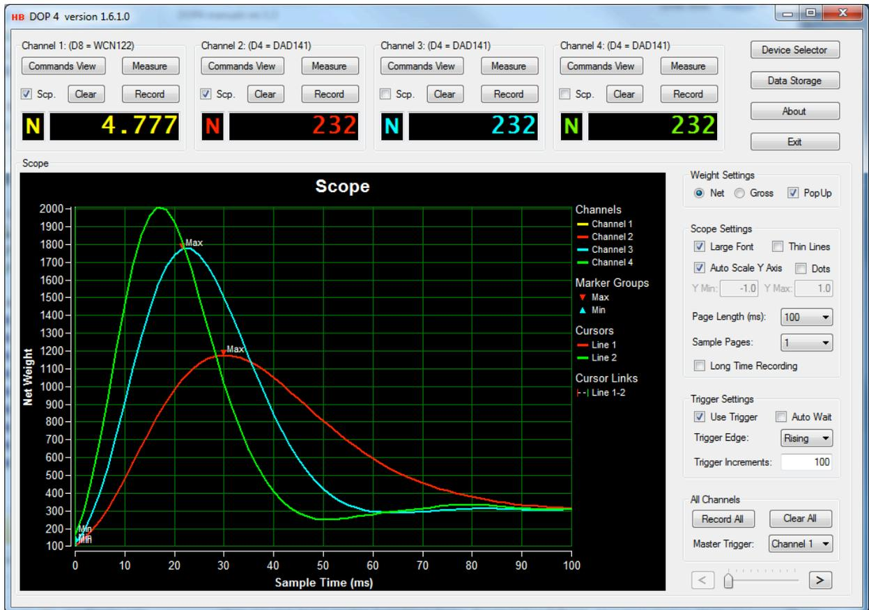
The main page consists of four channel groups from which recording, measurement and H&B device calibration can be controlled after one or more H&B devices are connected to the channels from the "Device Selector" dialog.
