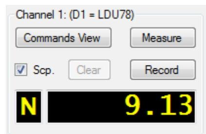
When the recording is started, the text of the "Record" button changes to "Stop". Select the "Stop" button for stopping the current load cell data recording.
