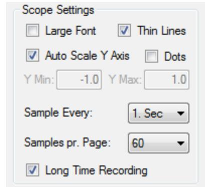
Define the sample interval for a given record session by selecting one of the preset sample interval values from the "Sample Every:" drop down box. The load cell data from the H&B device for recording will be polled by the defined time interval when the recording starts. In this case it's once every second.
