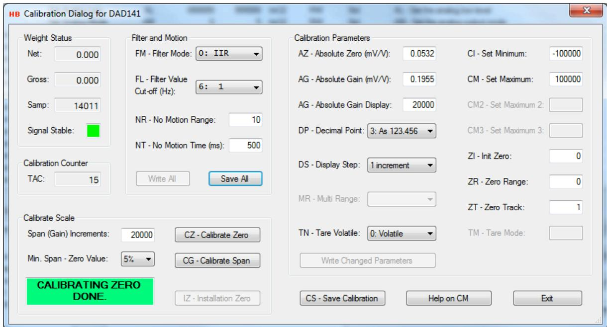
Before starting the calibration, be sure that the “Signal Stable” indicator is having a steady green indication when the load cell scale is in a steady state. If the “Signal Stable” indicator is red most of the time the scale is not steady enough to do a calibration.
