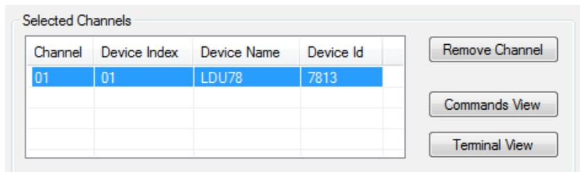
When checking the "Reload 'Selected Channels' at DOP 4 startup" check box, the selected H&B devices currently listed in the "Selected Channels" list view will be reloaded into the list view and opened, next time the DOP 4 application is started.
