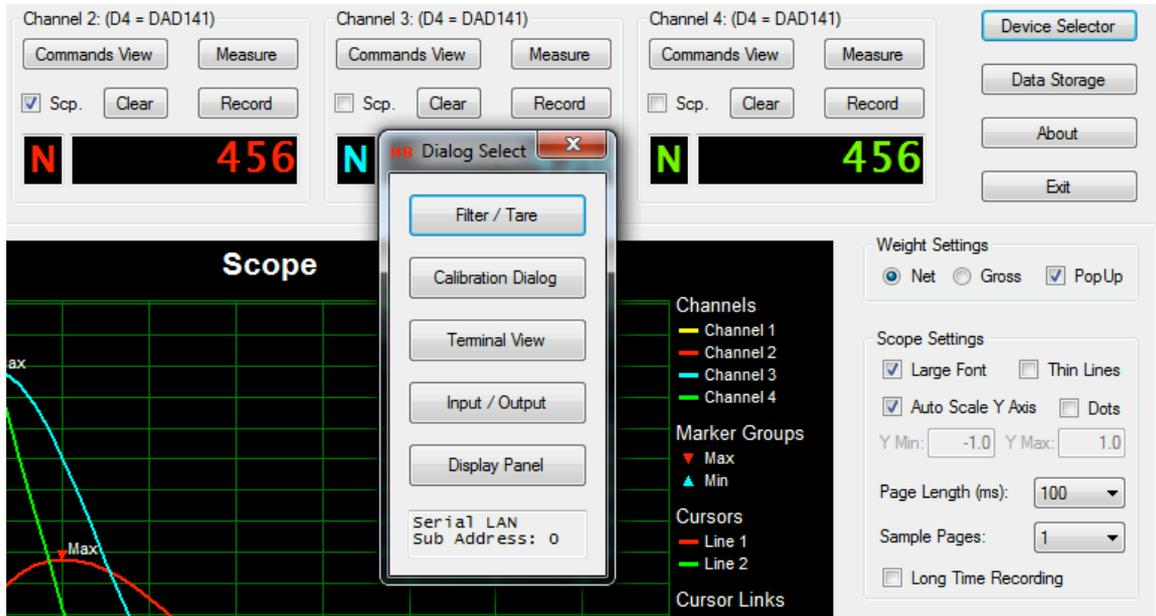
By having the "PopUp" checkbox unchecked, the "Filter / Tare" dialog can be reached by left clicking the mouse, having its cursor placed over an active channel weight display.
