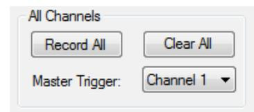
The load cell data recording from the two participating H&B devices to the scope display will start when the trigger condition for the device assigned to channel 1 is fulfilled.
