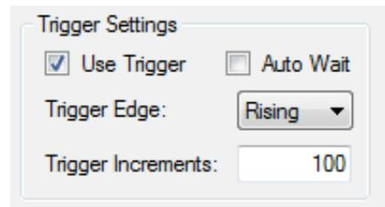
The increment value is e.g. the weight on the scale without the decimal point.
