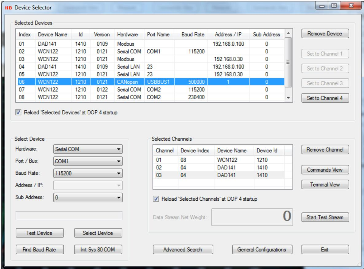
Select one or more H&B devices and assign them to one or more channels to be used in the main window, calibration and measurement dialogs.
