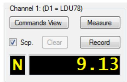
Load the scale with a weight higher than the specified increments value and the displaying of recorded load cell data on the scope display will start.
