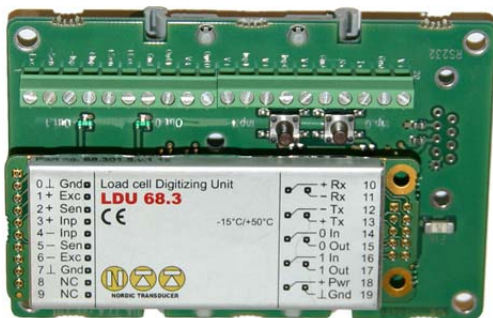
UA77.4 / 77.6 Board with screw terminals for I/O functions + 2 Input bottoms and + LED for output indication RS232 or RS485 output
