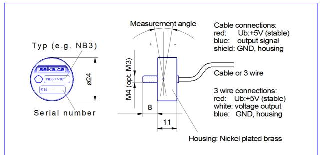
Attention! The supply voltage must not exceed 6 Volt and the polarity must not be reversed.
