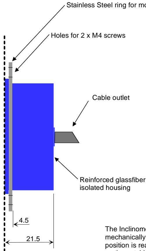
The Inclinometer housing can be turned mechanically inside the ring, when the wanted position is reached the 2 x M4 is tightened, and so the outside ring press on the housing so it is fixed in position.
