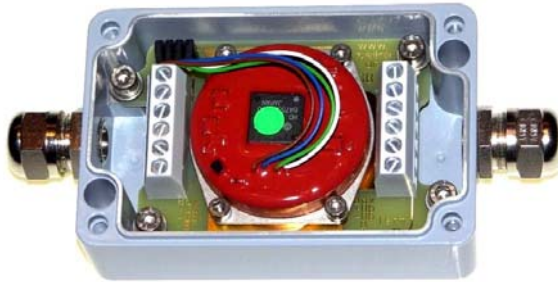
Sensor box containing one NG360 inclinometer with RS485 interface
