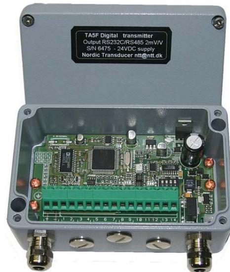
**TA5 Flash transmitter makes simple and cheap the remote transmission of the value sampled from strain gauges load cells to PLC, PC, recorders, remote indicator etc...**
